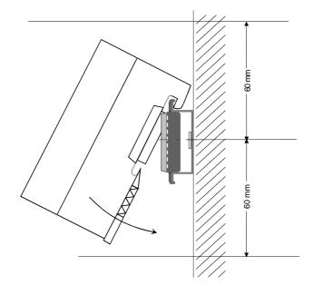
Installed and wired dimensions
