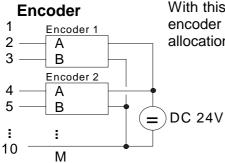
With this functionality 2 encoders can be connected. Configuring "Counter: encoder ..." 2 inputs (A, B) are switched to connect 1 encoder. Here the allocations for the respective  $2^{nd}$  input (B) are ignored.
